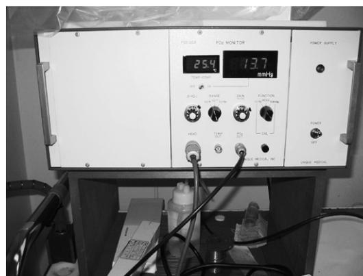
Fig 3. PO<sub>2</sub> Monitor-type PDG
